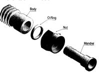
ing. The PRO-Crimp "F" connectors are available with nickel or gold plate finishes and in sizes for RG59/U, RG6/U and RG6/U quad shield cables.
